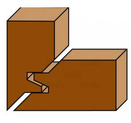
Klein® lock miter bits make perfect 45° locking miter joints with an easy process: the first board has to be run vertically while the second piece horizontally. If you want a simple joint, simply cut both pieces horizontally.
