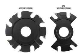
Adjustable grooving cutter with fixed blades in carbide (widia) for making thin precision grooves. Adjustable in height between 5mm and 9.5mm by means of spacer rings. Spacer rings sold seperately. Thanks to the tungsten carbide blades, this cutterhead cuts effortlessly through solid boards, hard and soft woods, MDF or laminated boards.
