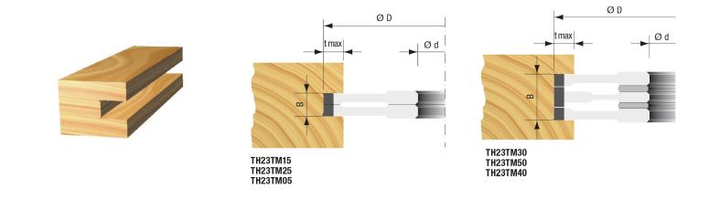
Adjustable cutterhead with reversible knives in high quality carbide metal (HW) for making thin precision grooves. Adjustable in height between 4mm and 7.5mm by means of spacer rings. Spacer rings included as standard. Thanks to the tungsten carbide blades, this cutterhead cuts effortlessly through solid boards, hard and soft woods, MDF or laminated boards.
