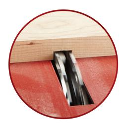
Adjustable groove blade set with adjusting rings that can be used on all sawing machines from the Itamac Panthera series. Can also be used on other machines equipped for dado blades. Note: Only a few machines on the market can be used with adjustable grooving saw blades. The thickness is fully adjustable up to 20.6mm.
