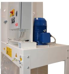
Dust extractors according to ATEX standards and for use in zone 22. Where the requirements of companies or prevention advisers in workplace zone 22 want to comply with the ATEX standards, these European dust collectors are an affordable solution. These powerful series are offered with Atex motor, Atex electrical cabinet, Atex filters and all Atex earthing and with all necessary certificates.
