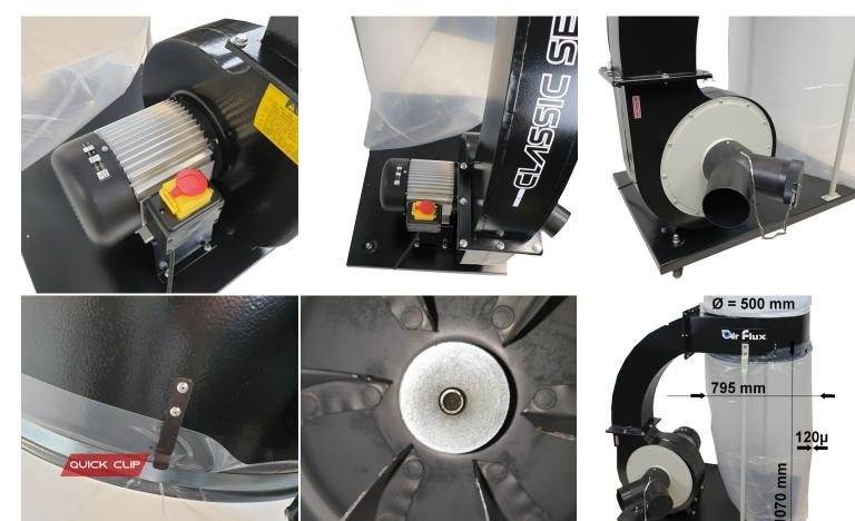
The Dusty 3000AF dust extractor has a fibre filter bag at the top that stops fine dust particles. Optionally there is also a Canister filter cartridge available that further purifies the air up to 0.5µm. This dust collector is equipped with a 2 HP induction motor with alu protection cap delivering an air flow of 2550m³/hour. Thanks to the wheeled base, the vacuum can easily be used throughout the entire workshop.
