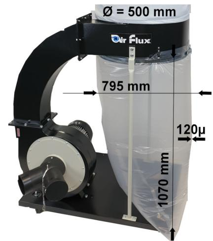
The Dusty 3000AF dust extractor has a fibre filter bag at the top that stops fine dust particles. Optionally there is also a Canister filter cartridge available that further purifies the air up to  $0.5\mu\text{m}$ . This dust collector is equipped with a 2 HP induction motor with alu protection cap delivering an air flow of  $2550\text{m}^3/\text{hour}$ . Thanks to the wheeled base, the vacuum can easily be used throughout the entire workshop.
