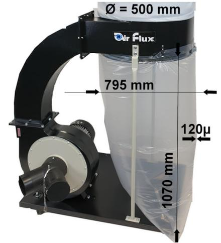
The Dusty 3000AF dust extractor has a fibre filter bag at the top that stops fine dust particles. Optionally there is also a Canister filter cartridge available that further purifies the air up to 0.5µm. This dust collector is equipped with a 2 HP induction motor with alu protection cap delivering an air flow of 2550m<sup>3</sup>/hour. Thanks to the wheeled base, the vacuum can easily be used throughout the entire workshop.
