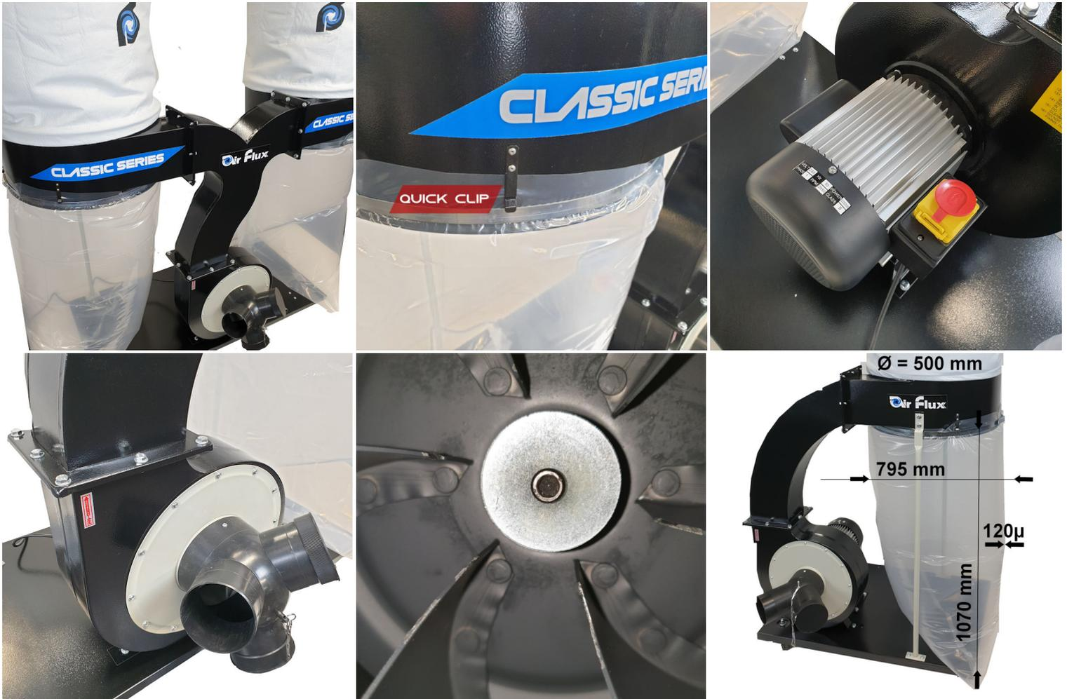
The Dusty 6000AF dust extractor has two fibre filter bags at the top that stops fine dust particles. Optionally there is also a Canister filter cartridge available that further purifies the air up to 0.5µm. This dust collector is equipped with a 3 HP induction motor with alu protection cap delivering an air flow of 3900m<sup>3</sup>/hour. Thanks to the wheeled base, the vacuum can easily be used throughout the entire workshop.
