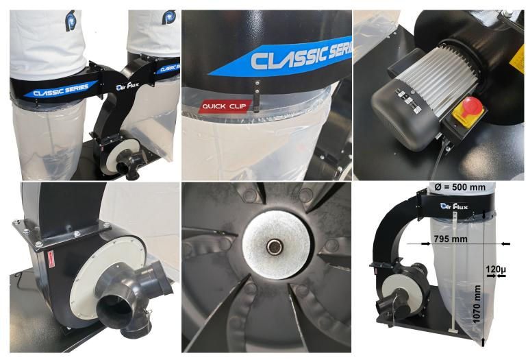
The Dusty 6000AF dust extractor has two fibre filter bags at the top that stops fine dust particles. Optionally there is also a Canister filter cartridge available that further purifies the air up to 0.5µm. This dust collector is equipped with a 3 HP induction motor with alu protection cap delivering an air flow of 3900m3/hour. Thanks to the wheeled base, the vacuum can easily be used throughout the entire workshop.
