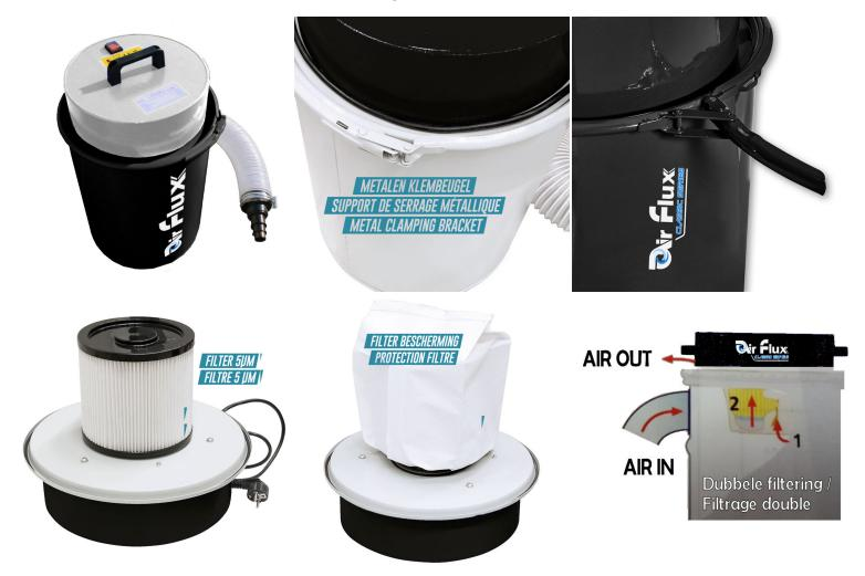
Compact dust extractor specifically designed for use in woodworking (sawdust, shavings and small shavings) in small workshops. Thanks to the large diameter of the extraction hose, this air extraction always maintains its air speed where conventional hoovers lose their speed. The bucket collector has a steel waste container with quick release closure and a capacity of 45 litres. Double filtration up to  $5\mu m$ . Multi adaptor available optionally.
