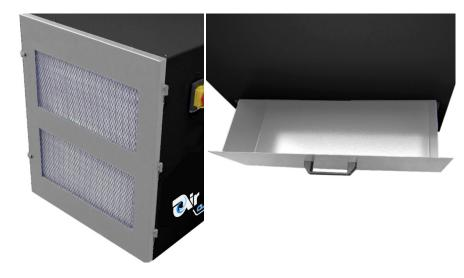
The Air Flux Dusty AF-1500MDC is a metal dust collector with powerful 230V or 400V, 2HP induction motor. The steel casing, combined with the 300mm blade impeller are able to deliver a reliable and efficient metal dust collecting. The dust is collected in a removable dust bin of 50L. The Dusty AF-1500MDC has two 100mm inlets and  $5\mu$ m galvanized air filters
