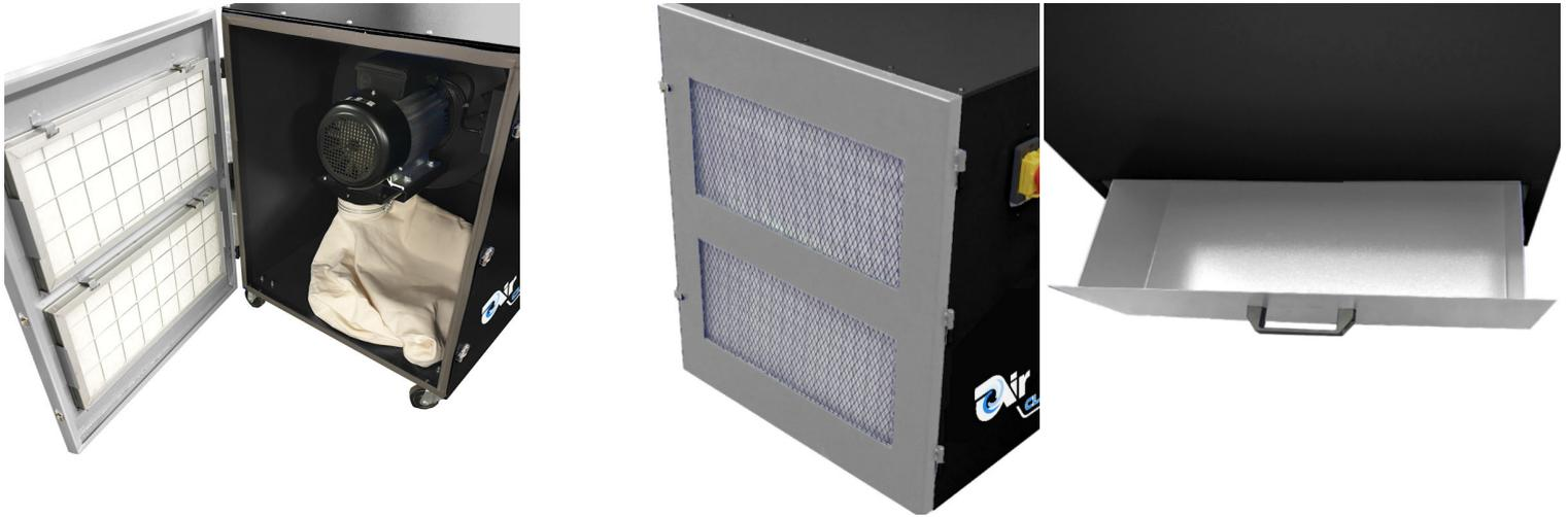
The Air Flux Dusty AF-1500MDC is a metal dust collector with powerful 230V or 400V, 2HP induction motor. The steel casing, combined with the 300mm blade impeller are able to deliver a reliable and efficient metal dust collecting. The dust is collected in a removable dust bin of 50L. The Dusty AF-1500MDC has two 100mm inlets and 5µm galvanized air filters
