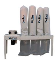
The Air Flux® Dusty AF-7000-DC is an industrial dust extractor with large collection capacity and low noise level. The sturdy sheet steel construction weighing 250 kg accommodates a three-phase 400 V motor, which generates an output of 7.5 HP and features a large propeller with a speed of 1440 rpm (instead of the usual 2880 rpm), which provides very quiet extraction. Furthermore, the vacuum cleaner is equipped with 8 filter bags (5 microns) above and 3 residual bags with a 600 mm diameter below.
