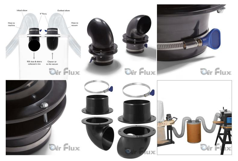
Separate large wood chips from your system before they reach your dust collector. A pair of plastic elbow and coupling components serve as input and output points when you install them at either end of a barrel, bin, or other receptacle you plan to use to capture large wood chips. This system prevents wear and tear on your dust collector and you don't have to empty it as often. The two coupling components fit a standard 100mm hose.
