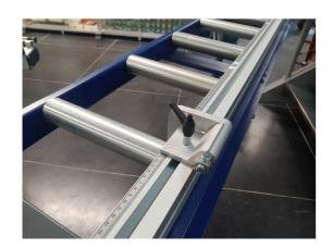
This aluminum profile of 3 meters can be used as a guide on our roller beds and tables.
