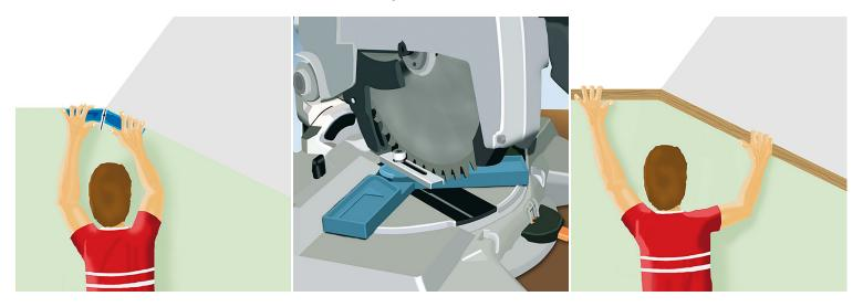
Virutex's 'Angle Copy' angle copier always ensures the correct angle without having to calculate or measure angles. Simply press the Angle Copy into the corner you are working in and the device will copy it. With the help of a button, you can affix the set angle so that the correct angle is always cut. Can be used in both inside and outside corners. Thanks to the protractor, you can also use the Angle Copy to manually indicate angles on your workpiece.
