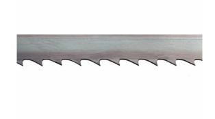
Bandsaw blade with length 1750mm for use on the TT250 band saw machine from Tendotools. This saw blade has 6 TPI (teeth per inch) and has a width of 6mm. This bandsaw blade in tempered steel "Flexback" is very suitable for multipurpose sawing. Use this saw ribbon for both wood and plastics. The teeth of the saw blade were given an additional heat treatment for increased hardness. This keeps the band very supple and increases your cutting comfort thanks to the hardness of the teeth.
