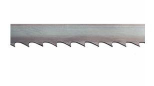
Bandsaw blade with length 2240mm for use on the TT312 band saw machine from Tendotools. This saw blade has 4 TPI (teeth per inch) and has a width of 10, 13mm or 16mm. This bandsaw blade in tempered steel "Flexback" is very suitable for multipurpose sawing. Use this saw ribbon for both wood and plastics. The teeth of the saw blade were given an additional heat treatment for increased hardness. This keeps the band very supple and increases your cutting comfort thanks to the hardness of the teeth.
