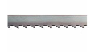
Bandsaw blade with length 3345mm for use on the TT400 band saw machine from Tendotools. This saw blade has 2 TPI (teeth per inch) and has a width of 25 or 32mm. This bandsaw blade in tempered steel "Flexback" is very suitable for multipurpose sawing. Use this saw ribbon for both wood and plastics. The teeth of the saw blade were given an additional heat treatment for increased hardness. This keeps the band very supple and increases your cutting comfort thanks to the hardness of the teeth.
