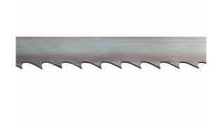
Bandsaw blade with length 3345mm for use on the TT400 band saw machine from Tendotools. This saw blade has 3 TPI (teeth per inch) and has a width of 20mm. This bandsaw blade in tempered steel "Flexback" is very suitable for multipurpose sawing. Use this saw ribbon for both wood and plastics. The teeth of the saw blade were given an additional heat treatment for increased hardness. This keeps the band very supple and increases your cutting comfort thanks to the hardness of the teeth.
