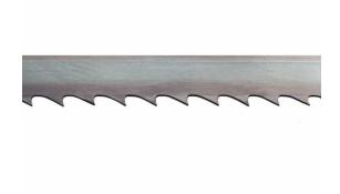
Bandsaw blade with length 3345mm for use on the TT400 band saw machine from Tendotools. This saw blade has 4 TPI (teeth per inch) and has a width of 10, 13mm or 16mm. This bandsaw blade in tempered steel "Flexback" is very suitable for multipurpose sawing. Use this saw ribbon for both wood and plastics. The teeth of the saw blade were given an additional heat treatment for increased hardness. This keeps the band very supple and increases your cutting comfort thanks to the hardness of the teeth.
