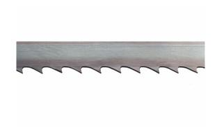
Bandsaw blade with length 3345mm for use on the TT400 band saw machine from Tendotools. This saw blade has 6 TPI (teeth per inch) and has a width of 6mm. This bandsaw blade in tempered steel "Flexback" is very suitable for multipurpose sawing. Use this saw ribbon for both wood and plastics. The teeth of the saw blade were given an additional heat treatment for increased hardness. This keeps the band very supple and increases your cutting comfort thanks to the hardness of the teeth.
