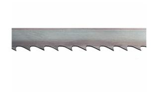
Bandsaw blade with length 3607mm for use on the TT500X band saw machine from Tendotools. This saw blade has 2 TPI (teeth per inch) and has a width of 32mm. This bandsaw blade in tempered steel "Flexback" is very suitable for multipurpose sawing. Use this saw ribbon for both wood and plastics. The teeth of the saw blade were given an additional heat treatment for increased hardness. This keeps the band very supple and increases your cutting comfort thanks to the hardness of the teeth.
