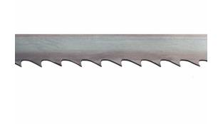
Bandsaw blade with length 3607mm for use on the TT500X band saw machine from Tendotools. This saw blade has 4 TPI (teeth per inch) and has a width of 13, 16 or 20mm. This bandsaw blade in tempered steel "Flexback" is very suitable for multipurpose sawing. Use this saw ribbon for both wood and plastics. The teeth of the saw blade were given an additional heat treatment for increased hardness. This keeps the band very supple and increases your cutting comfort thanks to the hardness of the teeth.
