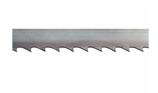
Saw ribbon with length 4590mm for use on the TT600 band saw machine from Tendotools. This saw blade has 2 TPI (teeth per inch) and has a width of 32mm. This bandsaw blade in tempered steel "Flexback" is very suitable for multipurpose sawing. Use this saw ribbon for both wood and plastics. The teeth of the saw blade were given an additional heat treatment for increased hardness. This keeps the band very supple and increases your cutting comfort thanks to the hardness of the teeth.
