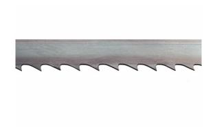
Bandsaw blade with length 4670mm for use on the TT50BS or TT61BS band saw machine from Tendotools. This saw blade has 4 TPI (teeth per inch) and has a width of 20mm. This bandsaw blade in tempered steel "Flexback" is very suitable for multipurpose sawing. Use this saw ribbon for both wood and plastics. The teeth of the saw blade were given an additional heat treatment for increased hardness. This keeps the band very supple and increases your cutting comfort thanks to the hardness of the teeth.
