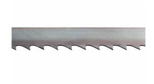
Saw ribbon with length 4590mm for use on the TT600 band saw machine from Tendotools. This saw blade has 4 TPI (teeth per inch) and has a width of 20mm. This bandsaw blade in tempered steel "Flexback" is very suitable for multipurpose sawing. Use this saw ribbon for both wood and plastics. The teeth of the saw blade were given an additional heat treatment for increased hardness. This keeps the band very supple and increases your cutting comfort thanks to the hardness of the teeth.
