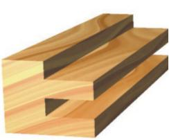
Belmash fixed groove cutter for both Belmash combination machines and spindle moulding machines. The groove cutter is used to produce rectangular grooves, to make quarters and to cut along the fibers in different types of wood. It can be used on woodworking machines BELMASH SDM2500, SDMR2500, CBS2400 or spindle moulders with shaft 30mm.
