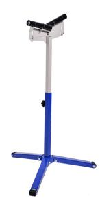
The Belmash RS-01 is invaluable when working with longer pieces of wood than the work table can support. This roller support provides a safe and easy way to work with these oversized pieces. Easy and convenient to use. Equipped with Teflon rollers to prevent damage to your workpiece. Both sides of the support can tilt by 45°. Height adjustable between 700mm and 1050mm.
