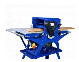
The thicknessing unit is an indispensable tool for thickness planing on the Belmash SDM2500 and makes it possible to obtain a workpiece of excellent quality. It has its own cutterblock that is driven via the motor of the SDM2500. With this unit you can plan thickness on the SDM2500 of 5-103mm and a planing width of 250mm.
