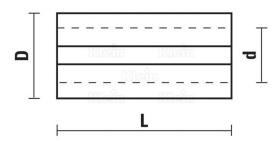
Bushing for shanks of router bits by Sistemi Klein. Use this bushing to use router bits with different shank diameters on your own machines.
