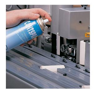
Significantly extend the life of your portable or stationary edge bander. The Virutex Cantspray is an antiadhesive spray without silicone. Suitable to treat all moving parts in your edge bander and prevent glue accumulation. Recommended to apply the Virutex Cantspray both before and after use of your machine for an optimal result.
