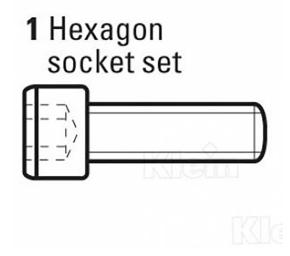
Spare cheese head screw to be used with the ball bearings for Sistemi Klein router bits.
