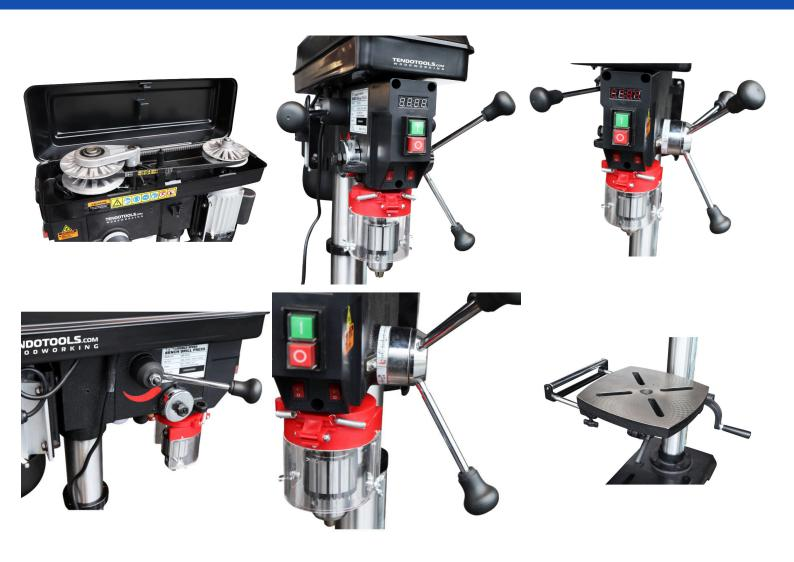
This unique column drill works with a variably adjustable speed (Variomatic). This variable speed feature allows you to set the right speed for any project (from 440 to 2850 rpm) without having to shift belts or open the gearbox.
