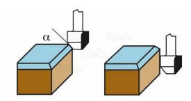
Bevel trim bits with combined cutting edges which allows to cut or machine laminated panels without replacing tools. The cutting edge is both straight and angled 45°. The bit can also be used for simple machining under angle.
