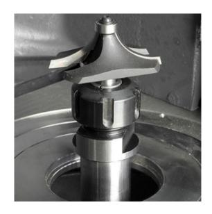
Concentric chuck with shank M14 to place on the spindle of your milling machine. To be used with spring collet T117 to mount router bits with shank diameter 8mm, 10mm or 12mm.
