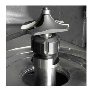
Concentric chuck with shank M16 to place on the spindle of your milling machine. To be used with spring collet T117 to mount router bits with shank diameter 8mm, 10mm or 12mm.
