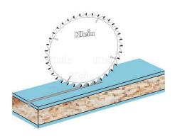
Conical scoring saw blade suited for cutting of double sided veneer, laminated boards, MDF and particle board To be used on panel sizing machines that allow the vertical adjustment of the scorer in relation to the panel sizing saw blade. Make sure to use the right amount of teeth to achieve optimal results of your project. A low number of teeth is suited for fast-paced and rough sawing. A high number of teeth calls for a lower operating speed but guarantees a clean cut.
