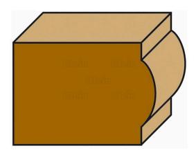
The hollow cutter quickly and easily mills convex edges or profiles on window sills, table edges, planks and making mouldings. Thanks to the cutting edges in high quality carbide metal, you can use this bit effortlessly on most types of wood. Pass multiple times when removing large quantities of material.
