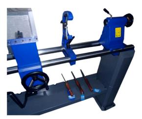
The TT1300 is a lathe for semi-professional use (Comfort Line), equipped with a powerful induction motor with an output of 1.5 hp and a copier. It has 4 speeds (500, 1000, 1950 and 2800 rpm), which are adjustable per belt. The lathe has a large capacity and is very stable while turning.
