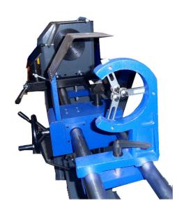
The TT1500 is a lathe for semi-professional use (Comfort Line), equipped with a powerful induction motor with an output of 1.5 hp and a copier. It has 4 speeds (500, 1000, 1950 and 2800 rpm), which are adjustable per belt. The lathe has a large capacity and is very stable while turning.
