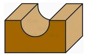
Thanks to these router bits you can cut a half-round groove on every kind of wood. They are still used to cut decorative grooves to break up large vertical surfaces and to adorn columns and edges. They are also often used to cut grooves for a better grip. For example for handles or drawers. Pass multiple times when removing large quantities of material.
