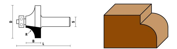
Round-over router bit to easily and quickly round corners. Increasing the working depth, you will obtain the classical "quarter-round" typical of dining table edges. Perfect finish of your project on different wood types thanks to the HW tungsten cutting edges.
