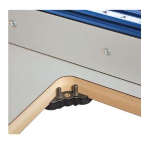
These levelling corners are the easiest way to install an insert in a home-made router table. There is no need for a supporting rabbet, and they have a unique design that allows them to be installed from below. They have eight adjustable contact points, four corner bolts for stability and placement tabs to facilitate installation.
