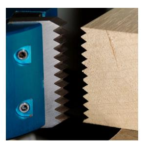
This cutter head for profile knives was designed for smaller milling machines with a bore diameter of 20mm.
