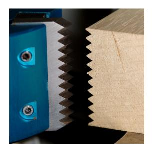
Cutter of height 90mm can be used on spindle moulding machines with a bore of 50mm. This cutter head is suitable to be used with all our profile knives of height 90mm. These high profiles knives are mainly used for milling panelling, cornices or roof profiles.
