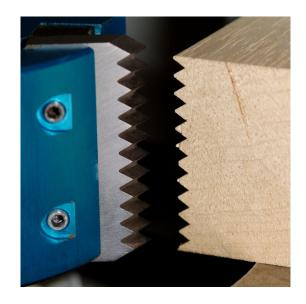
Universal cutter head which can hold almost every profile knive currently available on the market. This cutter head can carry both profile knives of height 40mm or 50mm as well as replaceable and reversible knives up to height 50mm. Thanks to the pre-cutters at the top and bottom, your work always has a clean finish. Also suitable for rabbeting.
