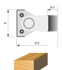
This adjustable bevel cutter head with high-quality tungsten carbide cutting edges gives you tremendous flexibility when making chamfers. The knives are adjustable on both sides between 0° and 70° in increments of 1°. Use the cutter head both for chamfering wood and board material. Thanks to the tungsten carbide blades, this cutterhead cuts effortlessly through solid boards, hard and soft woods, MDF or laminated boards.
