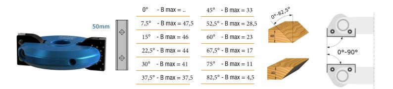
This adjustable bevel cutter head with high-quality tungsten carbide cutting edges gives you tremendous flexibility when making chamfers. The knives are adjustable on both sides between 0° and 90° in increments of 7,5°. Use the cutter head both for chamfering wood and board material. Thanks to the tungsten carbide blades, this cutterhead cuts effortlessly through solid boards, hard and soft woods, MDF or laminated boards.
